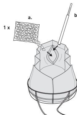
4. Tongranulat (a.) durch Öffnung einfüllen und Wasserstandsanzeiger (b.) einführen / Fill with expanded clay granulate (a.) through the opening and insert the water level indicator (b.)
